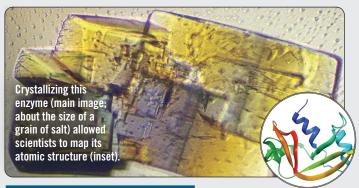
**How scientists created these images** Using chemistry, scientists prompted the protein sample to grow into a highly organized form called a crystal (over months). Then they fired X-rays through it. The X-rays bent in different directions upon hitting the individual atoms in the protein crystal, forming a dot pattern. Scientists used a formula to infer what 3D structure would cause that pattern. This process, X-ray crystallography, only works with specimens that *can* be crystallized.
